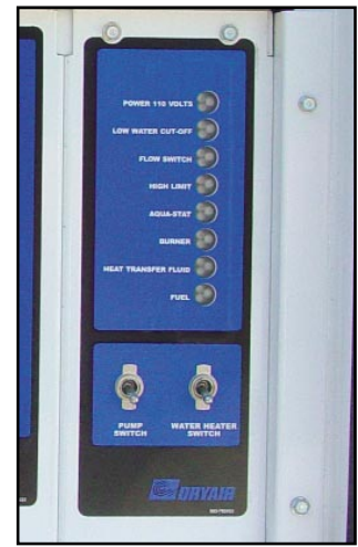
8-light diagnostic panel
