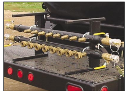
Fluid distribution manifold allows easy hook-up of hose
