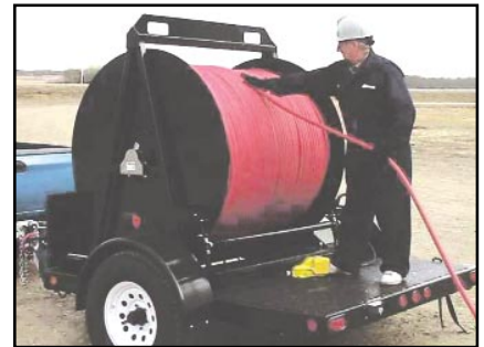
Reel capable of holding 6,000 feet of hose
