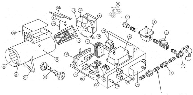
Port for measuring manifold pressure 1/4 FNPT
